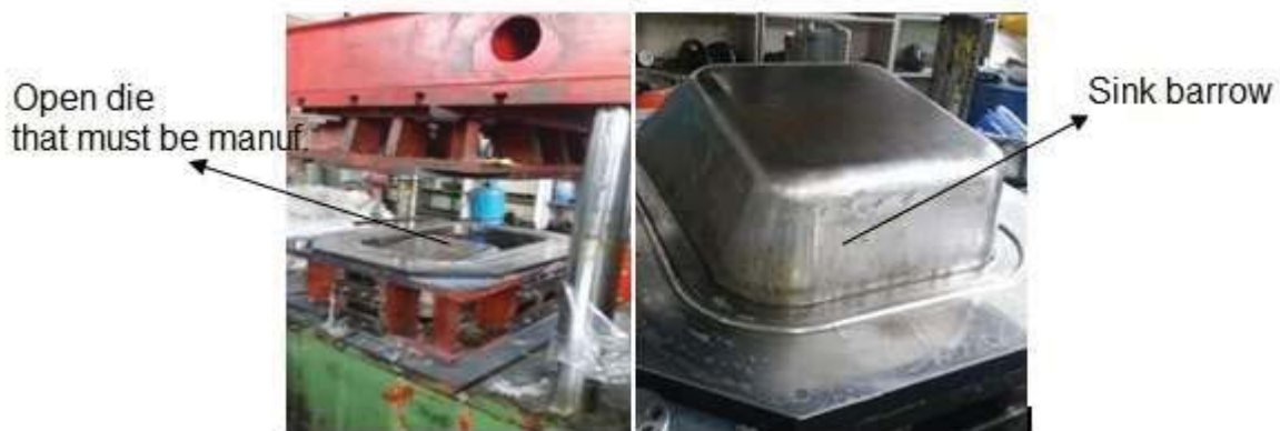
Figure 3. Press and open die tools, final shape
