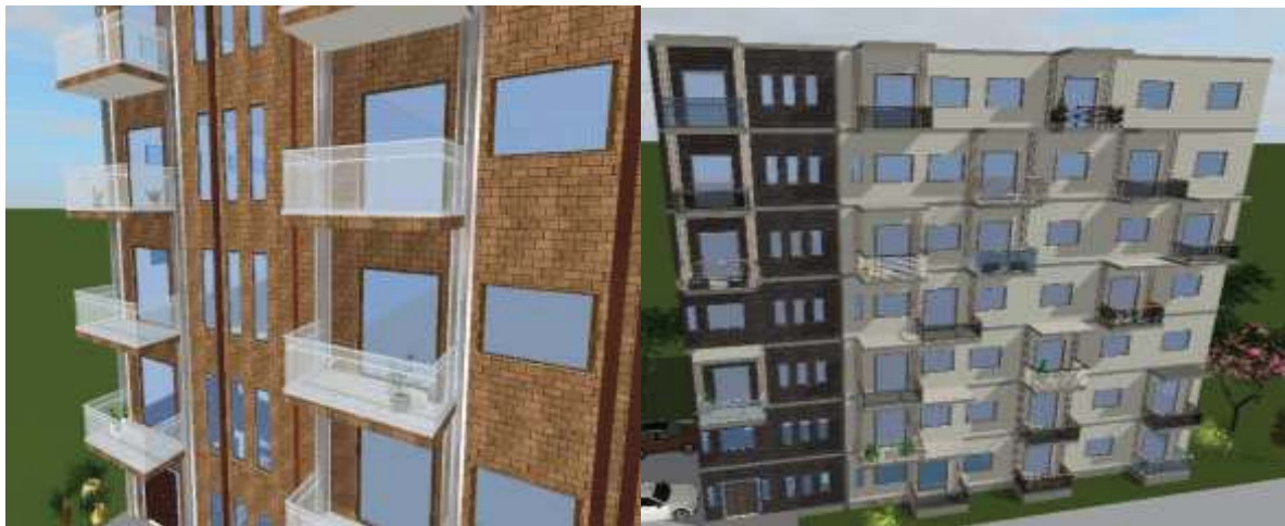
Figure 1: Prefabricated metal balcony applied to existent building
