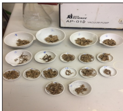
Figure 2. Final moisture content measurements (3 g samples) made for each technique applied
