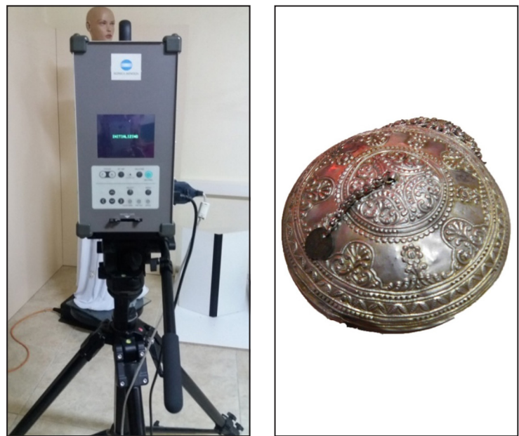
Figure 1. Konica Minolta Vivid 910 I 3D scanner (a), Silver plate folk object (b)
