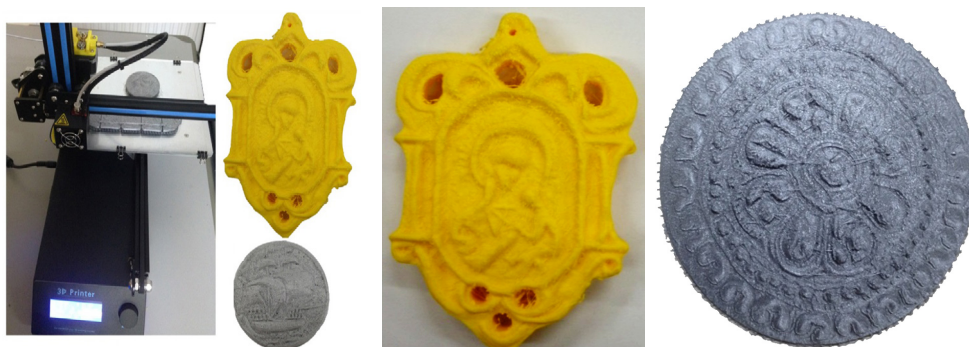
Figure 9. 3D Printed Objects in PLA 3D cartesian printer
