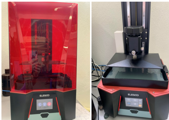
Figure 5. Preparing ELEGOO Saturn 2 for object printing
